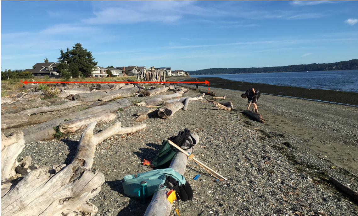
Figure 2.6. The log line is the distance between the log furthest from and closest to the water along a transect.
