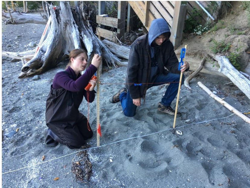
Figure 2.3. Field team measuring the beach profile using the 'string method'
